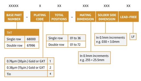
Note: 1. The total combined dimension for mating and solder side may not exceed 27mm
